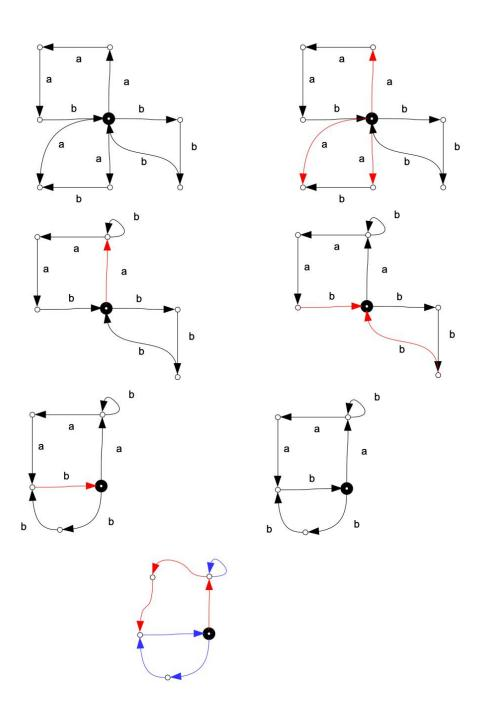
**Figure 1.1**: Flower automaton of  $W = \{a^{3}b, b^{3}, aba^{-1}\}$  and its foldings to obtain the Stallings graph of  $H = \langle W \rangle$ . Read the sequence of foldings top to bottom, right to left.
